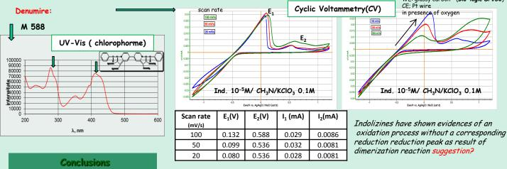
Design of an efficient synthesis method for new fluorescent indolizine compounds
